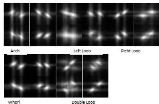
**Fig. 7.** Frequency transformation for each class (up left (Arch), up middle (Left Loop), up right (Right loop), down left (Whorl), down right (Double Loop))
