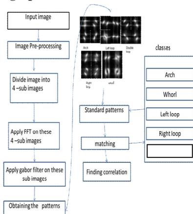
Figure 4. Fingerprint classification algorithm
