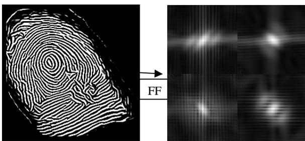
**Fig. 6.** Frequency domain representation for each sub image using 2D-FFT
