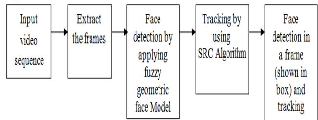
**Figure 1.** Block diagram of the proposed method
