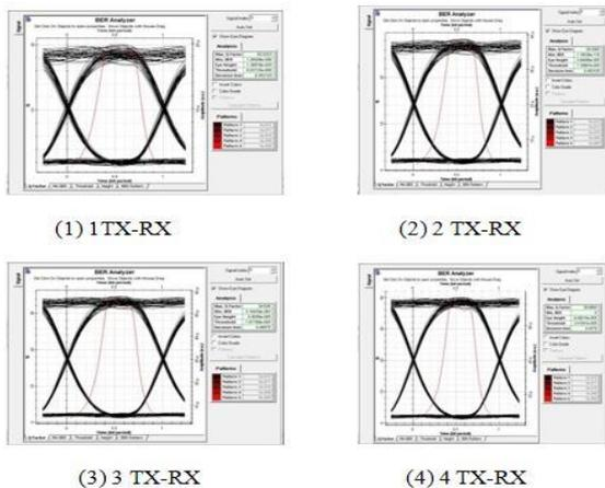
FIG 4 : BER Diagrams for receiver aperture = 8 cm
