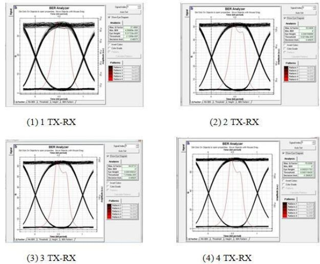
FIG 5 : BER Diagrams for receiver aperture = 15 cm
