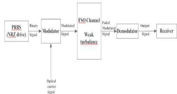
FIG 1: Free Space Optical Communication Link
