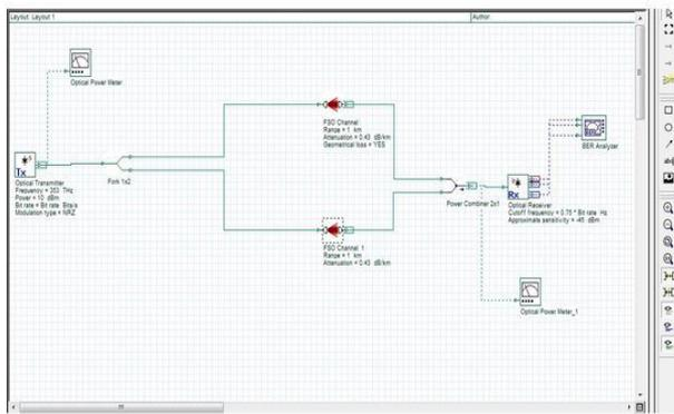
FIG 3: TX-RX FSO link simulation layout
