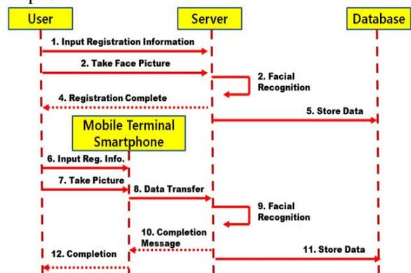
Figure. 3 Sequential Diagram of Registration
