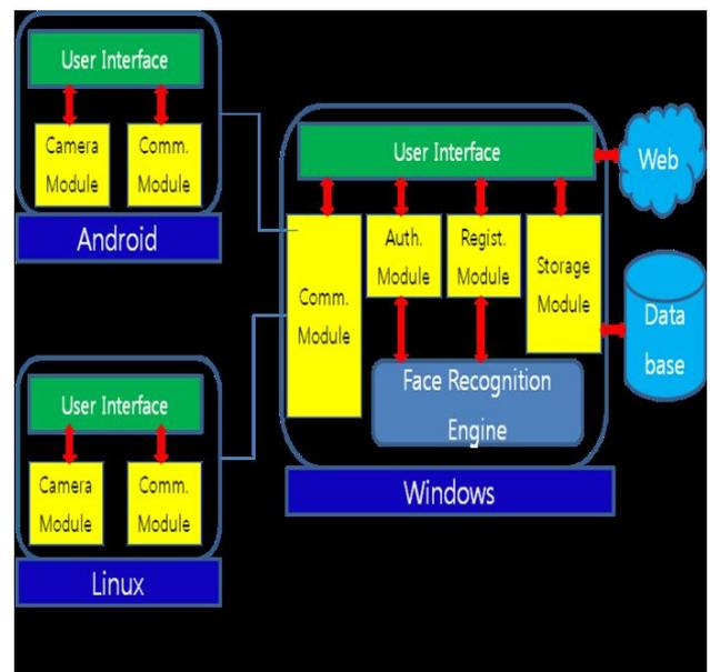
Figure.2 System Architecture
