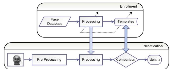
**Figure. 1** General Diagram of the Face Recognition System
