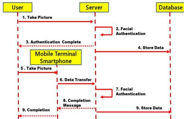
Figure 4. Sequential Diagram of Authentication
