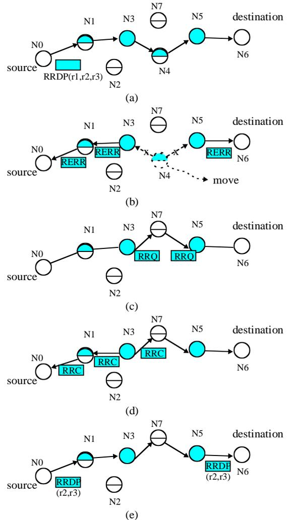
Fig. 5. Example of route backup process.
