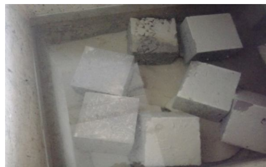
Figure 5. Curing Of Concrete
