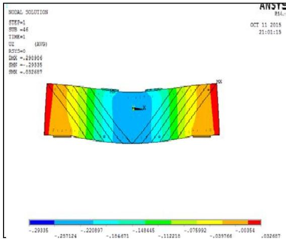
Figure 9 The Displacements In The Model After Non-Linear Finite Element Analysis For SB5A
