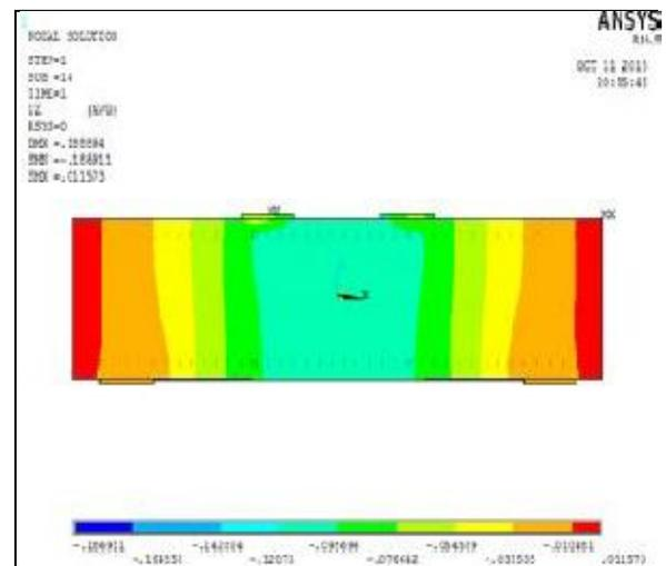
**Figure 7** The Displacements In The Model After Non-Linear Finite Element Analysis For SB3A
