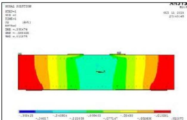
**Figure 4** The Displacements In The Model After Non-Linear Finite Element Analysis For CB
