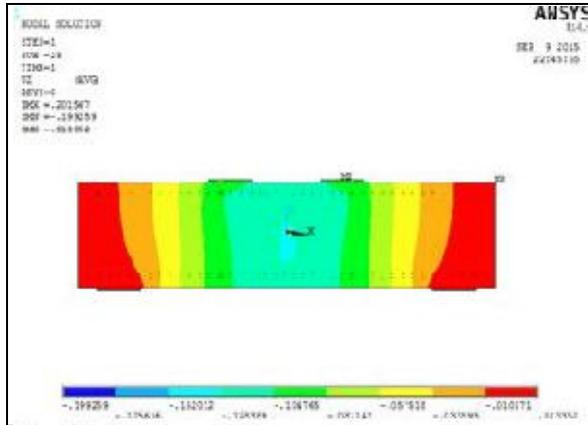
**Figure 3** The Displacement Of Palmyra Fibre
