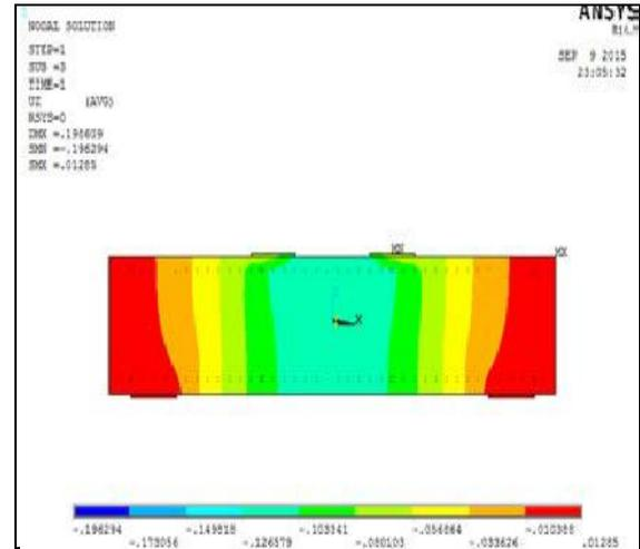
**Figure 6** The Displacements In The Model After Non-Linear Finite Element Analysis For SB2A
