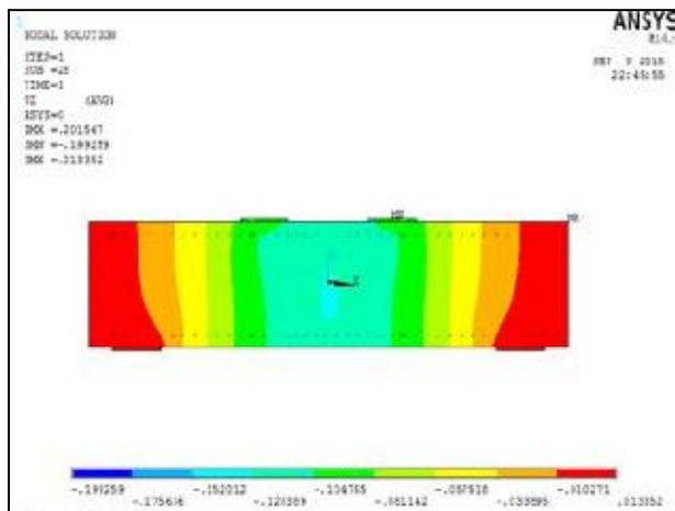
**Figure 5** The Displacements In The Model After Non-Linear Finite Element Analysis For SB1A
