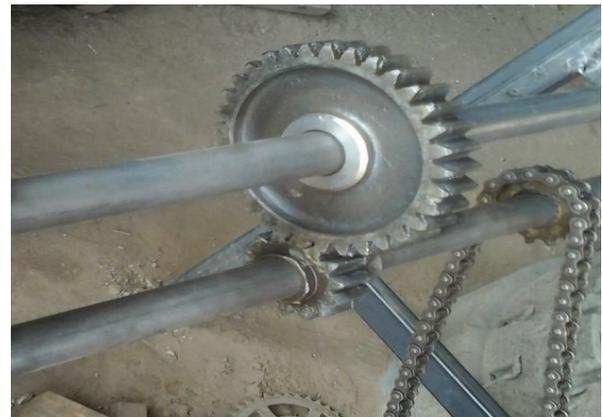
**Figure 11** Gear drive
