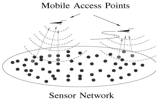
**Figure 2:** Sensor network with Mobile access points
