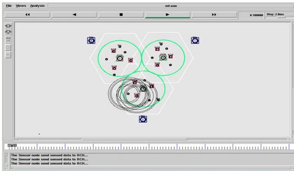
Figure 4: Sensor nodes transmitting the data to RCH
