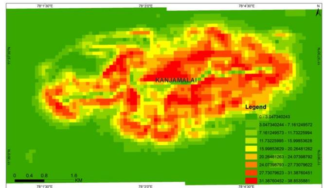
Figure 8 Slope angle of the Kanjamalai
