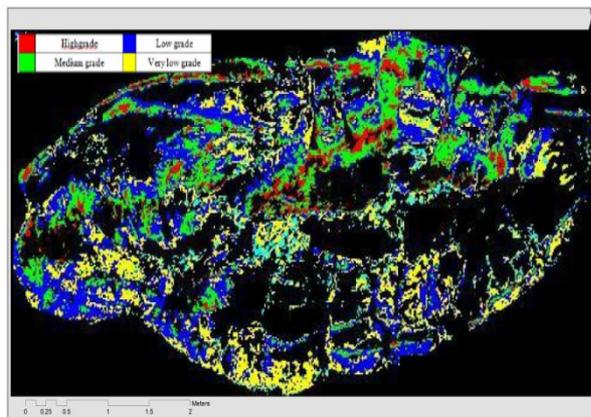
**Figure 13** Image showing iron ore grades in Kanjamalai
