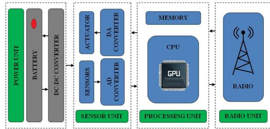
Figure 2 Schematic diagram of sensor node
