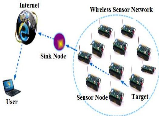
Figure 5 Spatial deployment and data transmission in WSN
