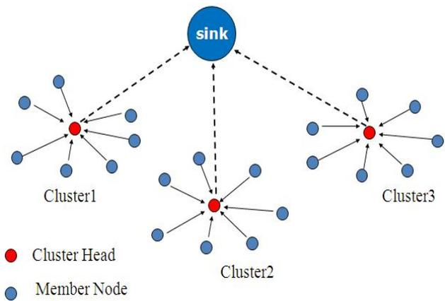
Figure 6 Block diagram of cluster topology
