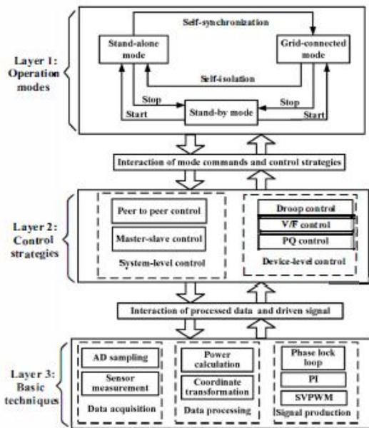
Figure 1 Control structure of PV microgrid.
