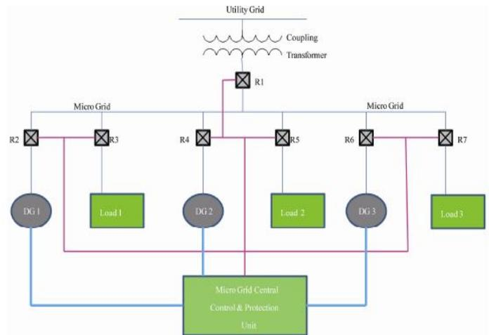
Figure 4 Topology of micro grid protection system
