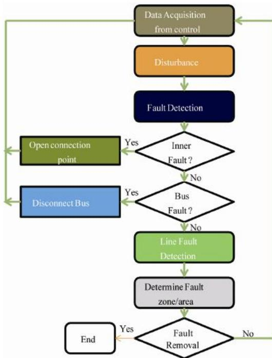
Figure 5 Fault mitigation technique of micro grid
