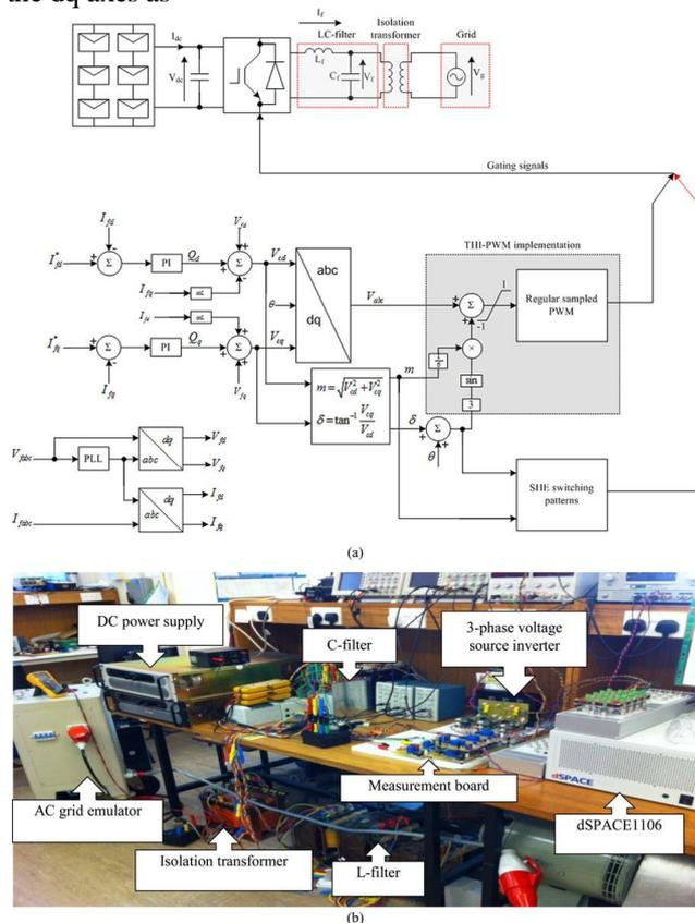
**Figure 3** (a) Schematic diagram of a grid-connected PV inverter with SHE and THI PWM using a dSPACE1106 hardware implementation and (b) p.u. scaled-down test rig of a multimewatt PV inverter prototype.
