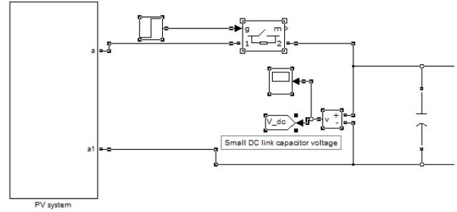
Figure 6 PV and Boost DC/DC Converter
