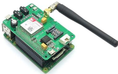
Fig-4 GSM Module With Raspberry pi 3.
