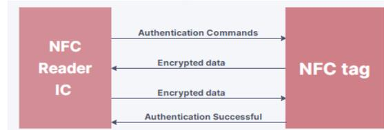
Figure 4 Authentication model of NFC
