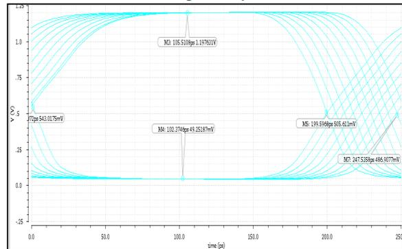
Figure 12: Simulated eye diagram for Hybrid VCO
