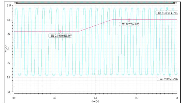
Figure 5: simulated Output Waveform of Hybrid VCO
