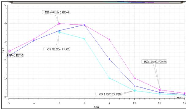
Figure 7: simulated and Measured Kvco Gain Vs control voltage
