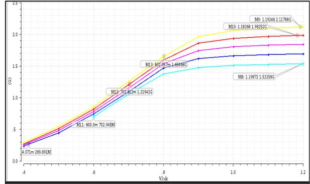
Figure 10: Variation of Frequency with different supply voltage
