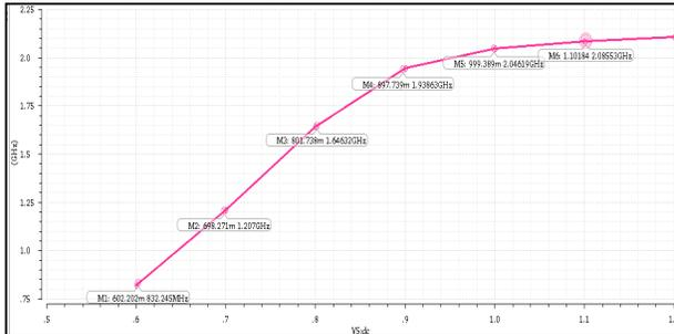
Figure 8: Frequency variation with varying control voltage On increasing the temperature the frequency of oscillation decreases. Figure 10 displays the frequency variation as a function of control voltage and supply voltage. From the obtained results the frequency of oscillation is directly proportional to supply Voltage. For supply of 1V frequency is 1.5GHz and Increases to 2.61GHz for the supply of 1.2V.
