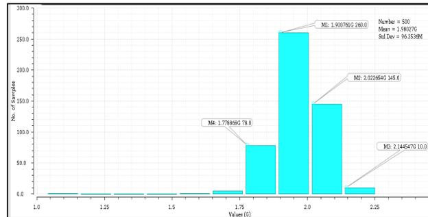
Figure 6: Histogram plot for oscillation frequency obtained from monte carlo simulation
