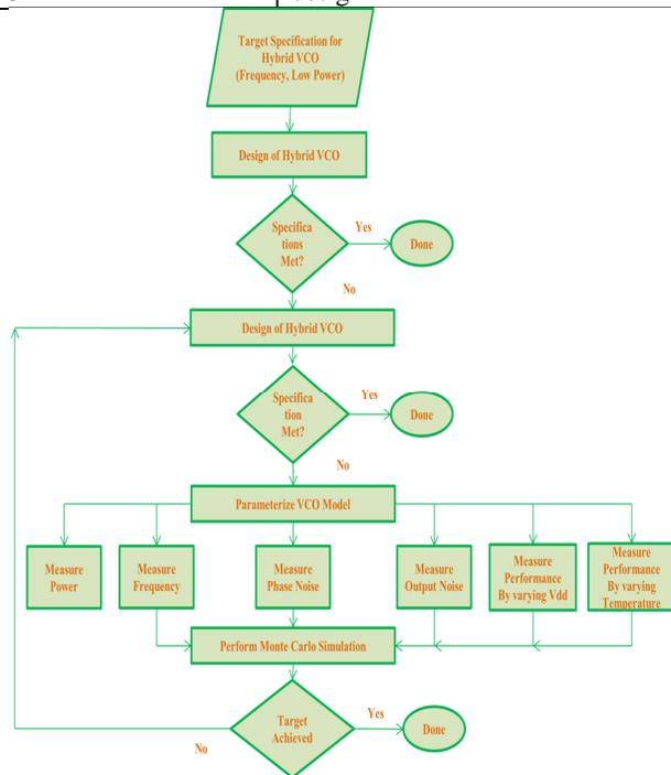
Figure 2: Flow chart of proposed Hybrid VCO
