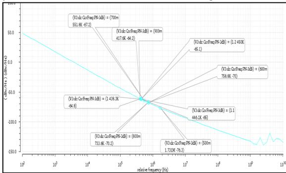
Figure 14: Simulated and Measured Phase Noise of Proposed Hybrid VCO
