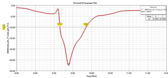
**Figure 6** Return Loss (dB) plot of B-sandwiched radome integrated with 2x2 MPAA
