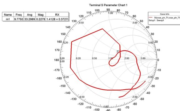
**Figure 8** Smith Chart of B-sandwiched radome integrated
