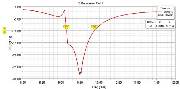
**Figure 4** Return Loss of 2x2 MPAA
