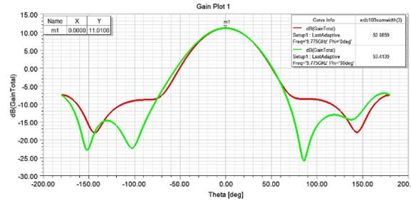
**Figure 3** Gain (dB) plot of 2x2 MPAA
