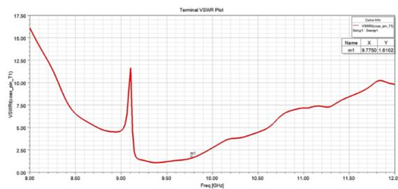
**Figure 7** VSWR plot of B-sandwiched radome integrated with 2x2 MPAA
