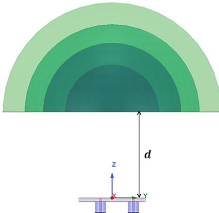
**Figure 2** B-sandwiched radome with feed element
