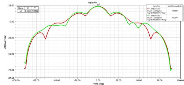
**Figure 5** Gain (dB) plot of B-sandwiched radome integrated with 2x2 MPAA
