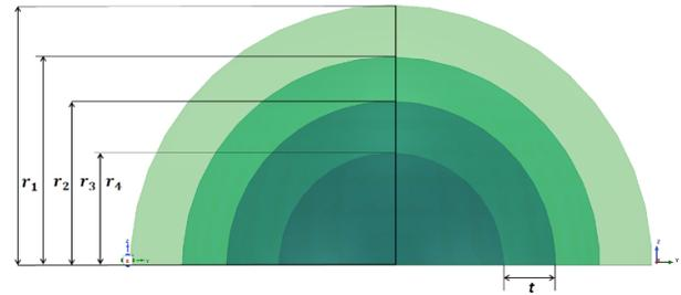
Figure 1 B-sandwiched radome (Front view)
