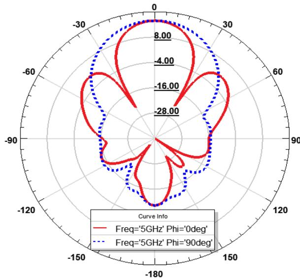
Fig. 4: Radiation pattern of 4x2 MPAA with power divider
