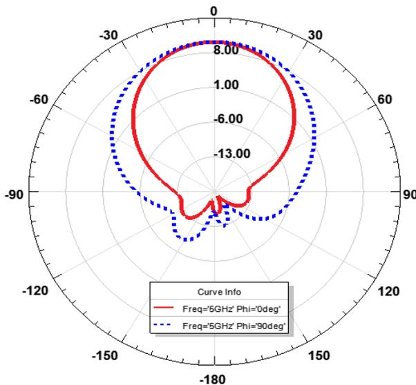
Fig. 2: Radiation pattern of 1X2 sub-array with power divider
