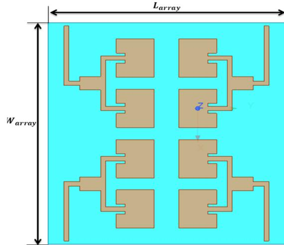
Fig. 3: 4X2 RMPA array Schematic
