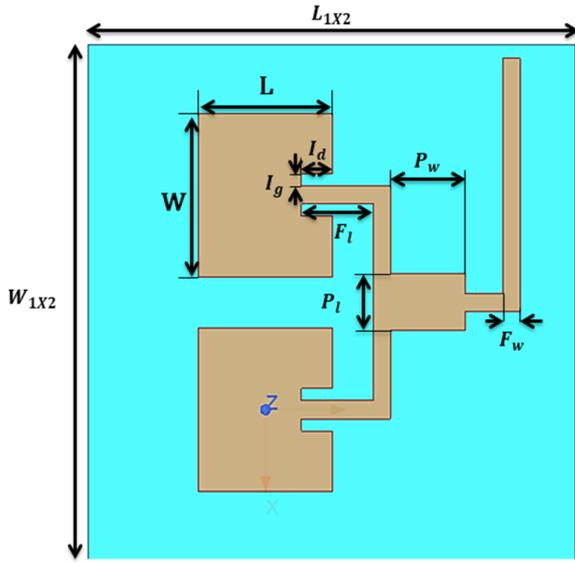
Fig. 1: 2X1 RMPA sub-array Schematic
