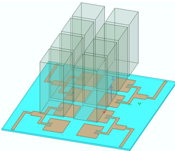
Fig. 5: 4x2 RMPA array with RDRA Schematic (isometric view)
