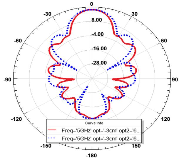
Fig. 6: Radiation pattern of 4x2 MPAA with power divider
