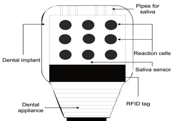
**Figure 1** Dental implant with saliva sensor and RFID tag inside
