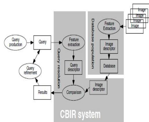
Figure 1: Shows the Content Based Image Retrieval System.
