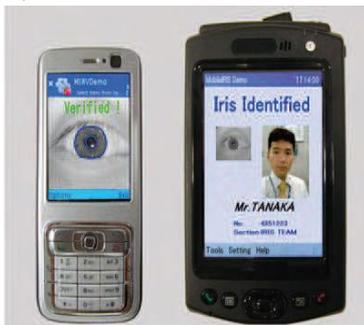
**Figure 10.** Iris recognition technology for mobile terminals. [8]
