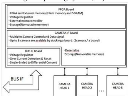
Fig. 3: System Architecture of HP-IMAP-EO
