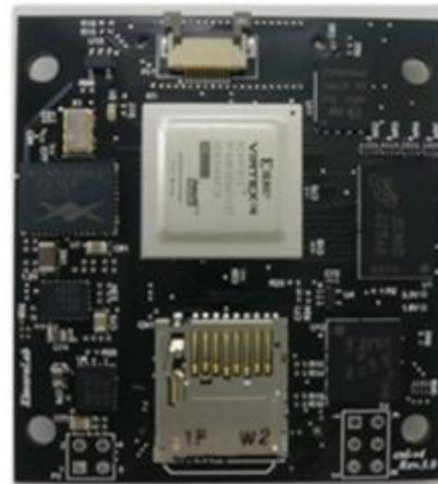
Fig. 4: FPGA Board
