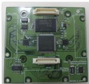
**Fig. 5:** Camera Interface Board
