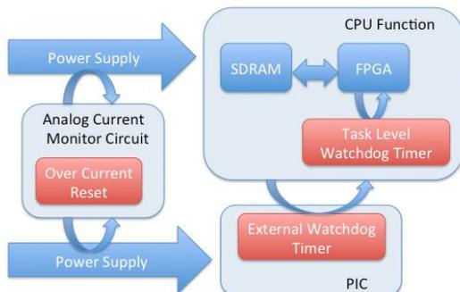
**Fig. 2:** Concept of Hierarchical Monitoring System
