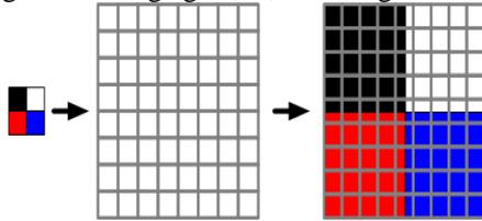
Figure 1 Example of Up sampling an Image by a Non-Integral Factor
