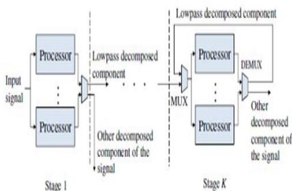
**Figure 5** Block diagram of pipeline architecture
