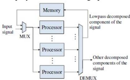
**Figure 4** Block diagram of parallel-processor architecture
