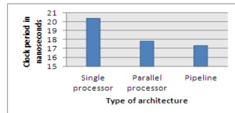
**Figure 6** Graph illustrating the computation time for three types of architectures.
