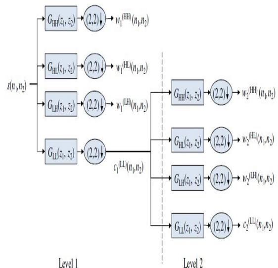
**Figure 2** Representation of the computation of a 2-level 2-D DWT based on non-separable approach
