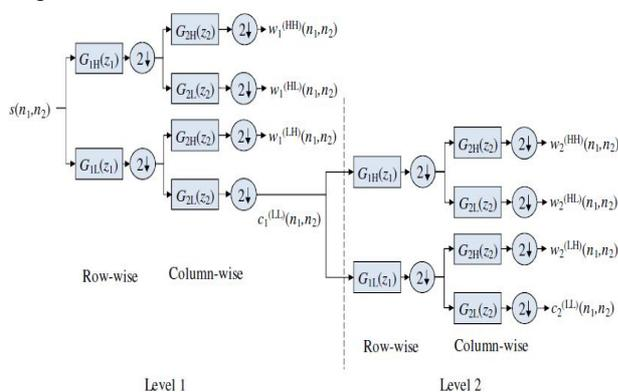
**Figure 1** Binary tree representation of the computation of a 2-level 2-D DWT based on separable approach
