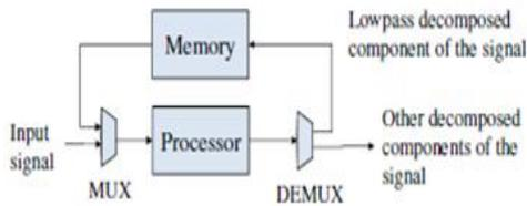
**Figure 3** Block diagram of single-processor architecture
