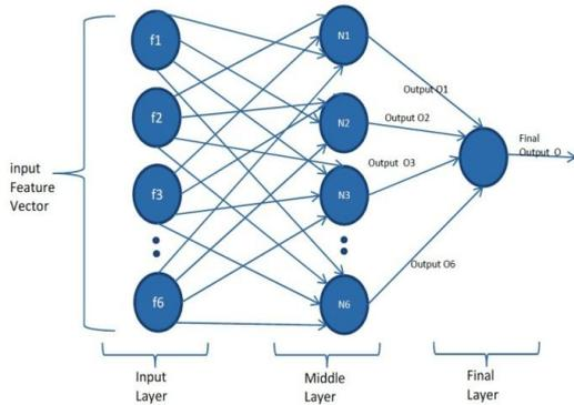
Figure 2 Learning Process of Multi-Layer Artificial Neural Network
