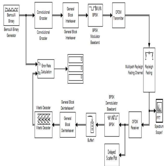
Fig 2. Simulink model of DAB transmitter and receiver.
