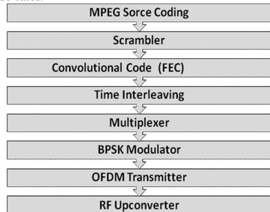
**Fig1.**DAB functional diagram of transmitter
