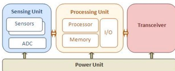
**Figure 3.1** Architecture of a Sensor Node
