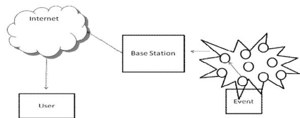
**Figure 3.2** The Communication Architecture of Sensor Network
