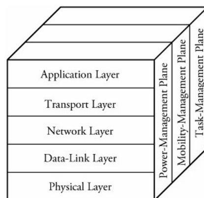
**Figure 3.3** The Sensor Networks Protocol Stack
