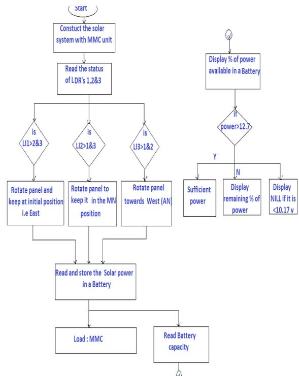
**Figure.4:** Flow Chart of Solar Power System for MMC
