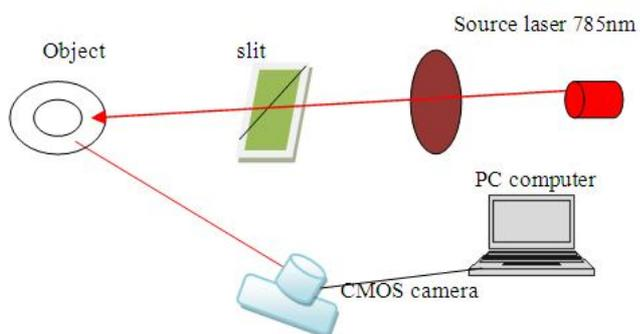
**Figure 3** Schematic of the experimental setup for digital hologram using CMOS camera .
