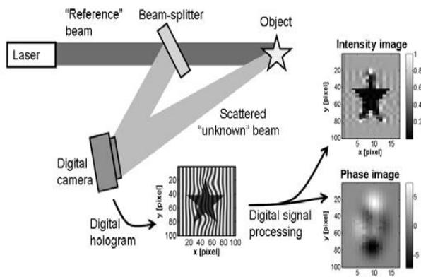
**Figure 1** Setup for off-axis digital holography, showing the recording and reconstruction steps.
