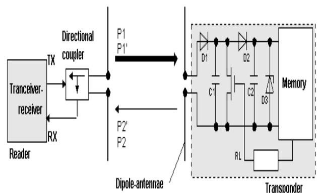
**Figure 4** Load Modulation techniques for data transfer
