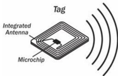
**Figure.1** RFID tag with antenna and Chip
