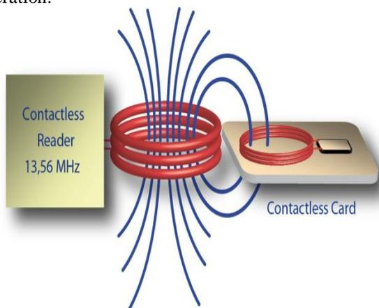
**Figure 2** Inductive Coupling RFID System
