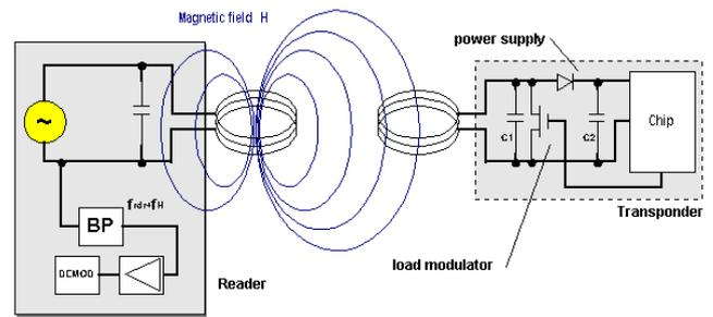
**Figure 3** Load Modulation techniques for data transfer
