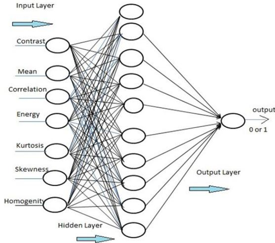
Fig. 7 Structure of Artificial Neural Network
