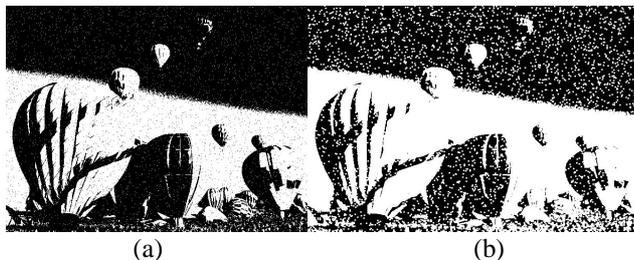
**Figure 3** Example of the erosion: a. Original image A; b. The result image:  $A \ominus SE$ .
