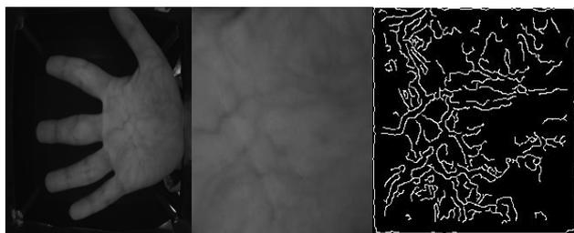
**Figure 7** Illustration of image enhancement: (a) The original image (b) Extraction of ROI (c) Extraction of Palm vein pattern
