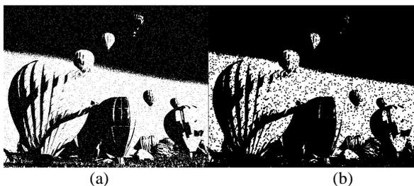
**Figure 2** Example of the dilation: a. Original image A; b. The result image:  $A \oplus SE$  [14].
