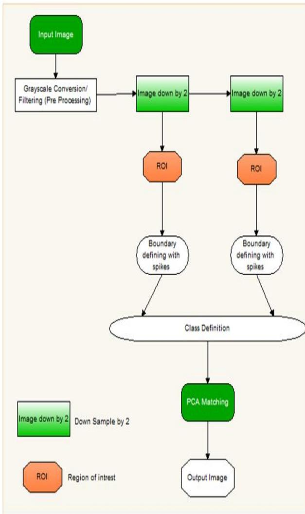
Fig.2: Flow Sequence of the Proposed Design Methodology
