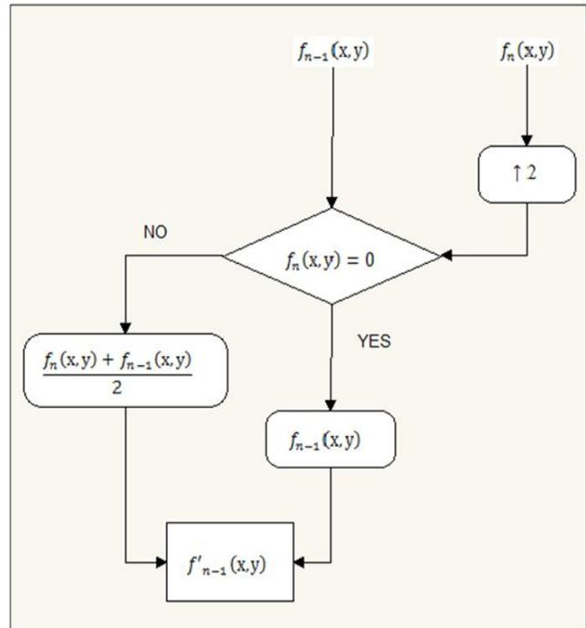
Fig. 3: Flow Chart for Obtaining Segmented image
