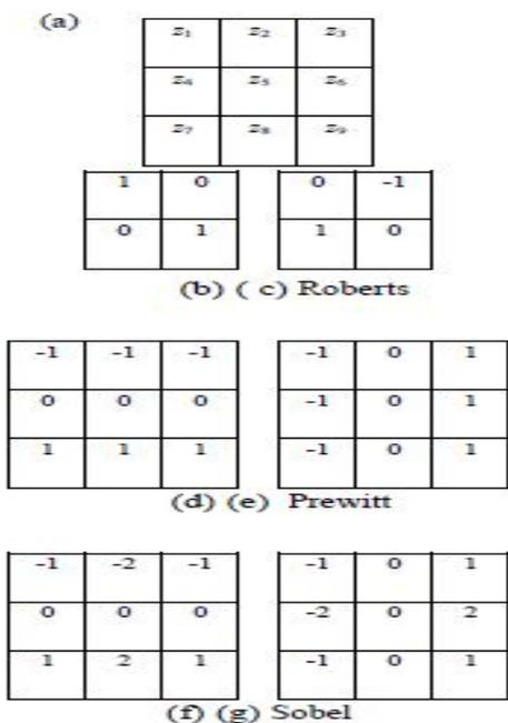
Fig. 3.1 A 3 x 3 region of an image (the z's are gray-level values) and various masks used to compute the gradient at point labeled  $z_5$ .
