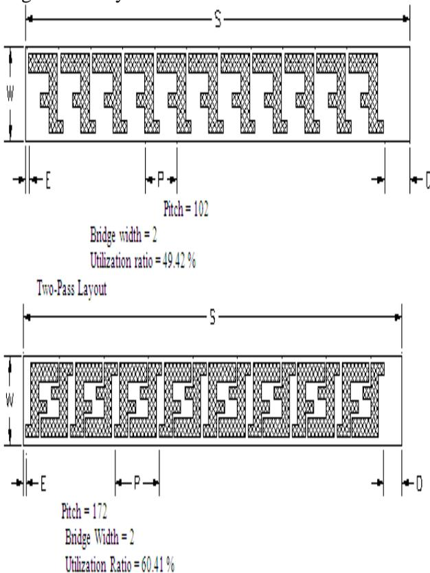
**Fig.(3-a)** Representative illustration for determining the number of blanks in a strip.
