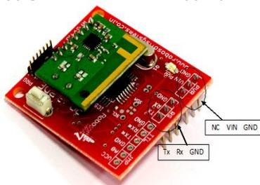
Figure 2: RF Transceiver
