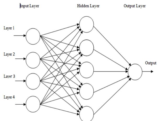
**Fig2.** General structure of Multilayer Perceptron Neural Network
