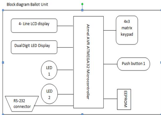
**Figure 2:** Block diagram of Ballot unit
