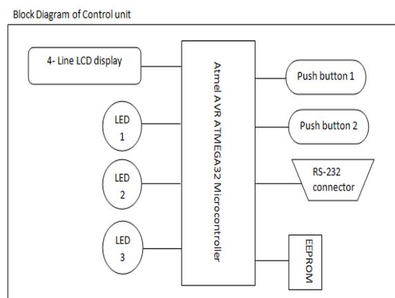
Figure1: Block diagram of Control unit
