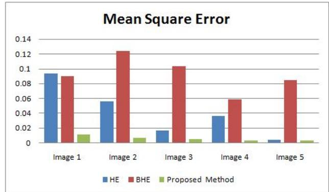
**Fig. 8:** Graphical Comparison of Proposed method with HE and BHE on the basis of MSE
