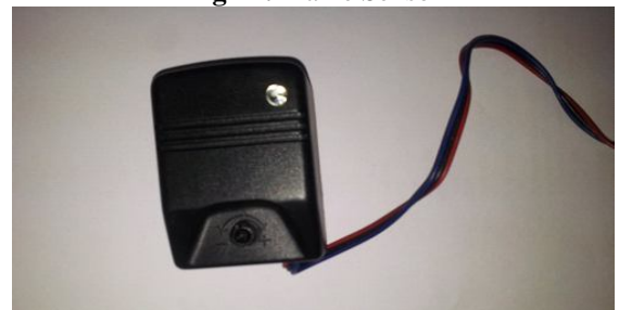
Fig 12: piezoelectric transducer/Knock Sensor
