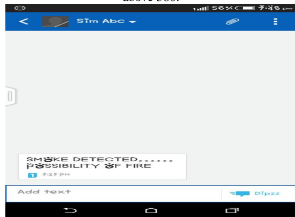
Fig 14: SMS received after the smoke detected on the registered mobile.
