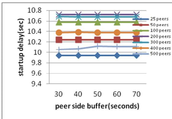
**Figure 3:** Impact of peer side buffer over startup delay
