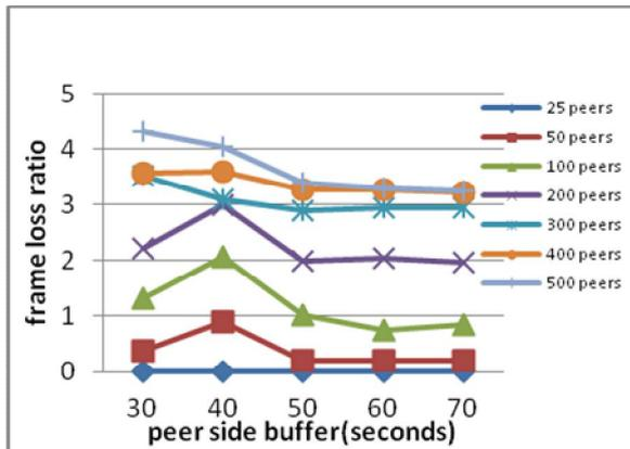
**Figure 2:** Impact of peer side buffer over frame loss (Non Cluster)
