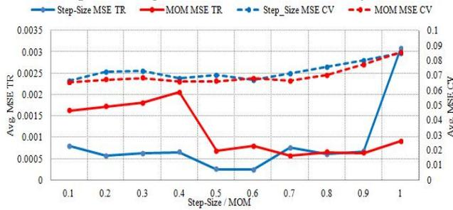
**Fig.6.** Variation of Average Minimum MSE with step size and momentum rate of Output layer and output layer
