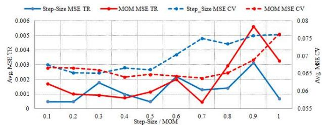
**Fig.7.** Variation of Average Minimum MSE with step size and momentum rate of Hidden layer and output layer
