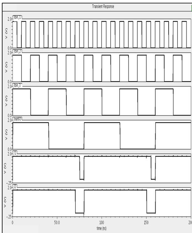
**Figure 5 a)** Simulation Result of Binary to Thermometer Decoder
