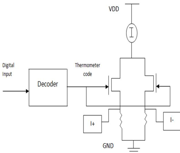
**Figure 2** Design of Thermometric type of DAC
