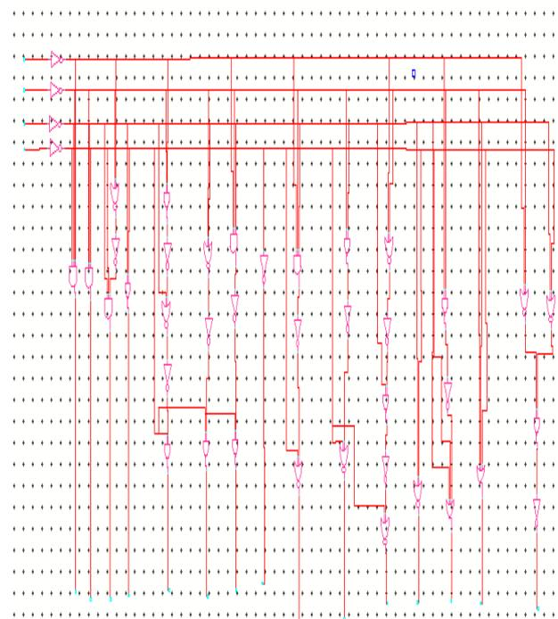
**Figure 4** Four to Fifteen Binary to Thermometer Decoder
