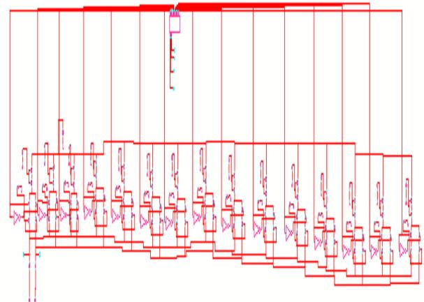
**Figure 3** Schematic Design of Thermometer type of DAC
