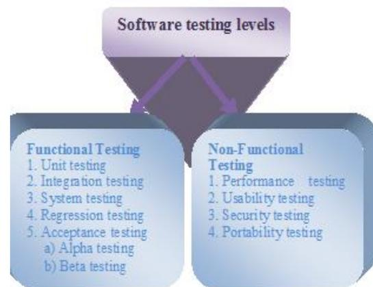
Figure 2 Software Testing Levels
