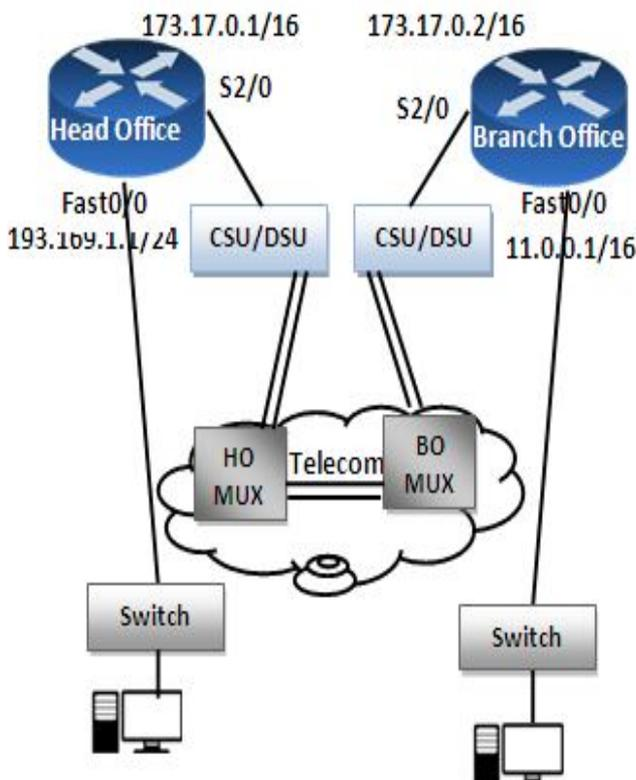
Fig. 1.0 Shows WAN Design (Head office to Branch Office Connectivity)
