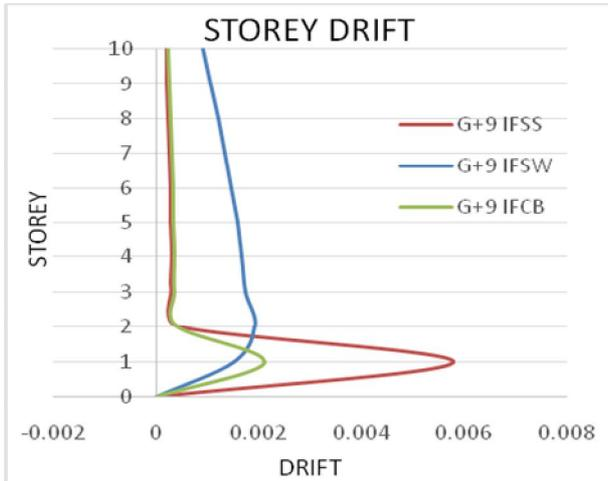
**Figure 7** Drift Vs Storey
