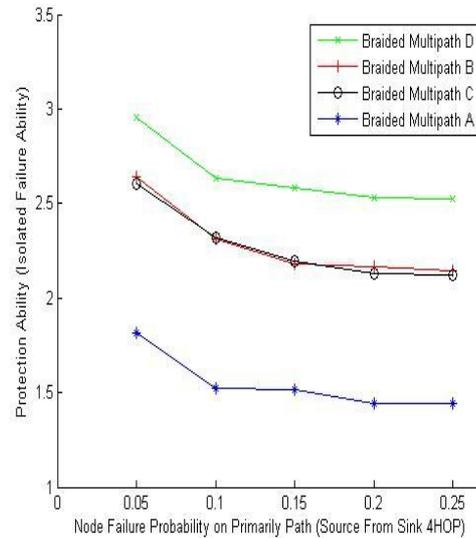
**Fig. 7: AP vs. node failure probability**
