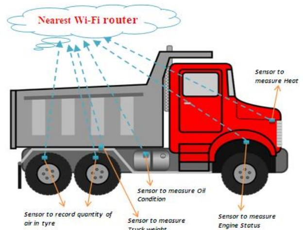
**Figure 4:** Sensor network to manage Vehicle through IoT
