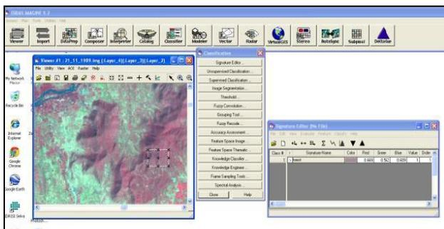
FIGURE 5 Shows How To Edit Signature From Satellite Image In Erda
