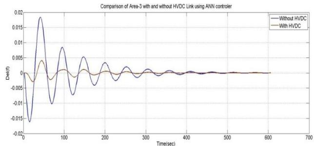
Figure 6: Area-3 del f Comparison with and without EHVAC/HVDC link
