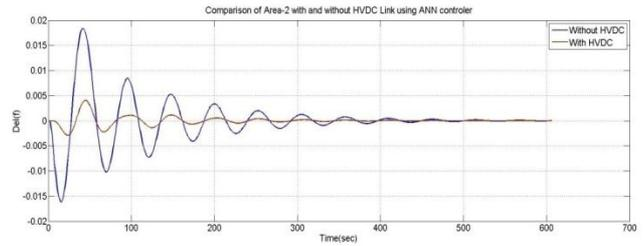
Figure 5: Area-2 del f Comparison with and without EHVAC/HVDC link
