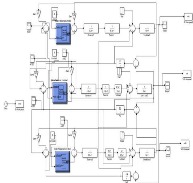
**Figure 2: Three area Power system with neural network without HVDC link**
