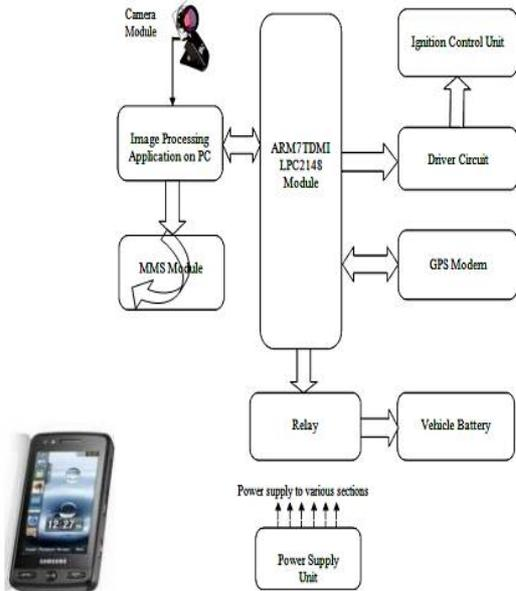
**Fig 1:** Block Diagram of Automotive Security System
